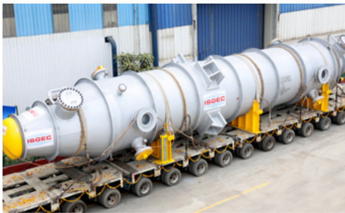
Heat Exchanger with Internal Bore Welding (Licensor's Proprietary Equipment)
